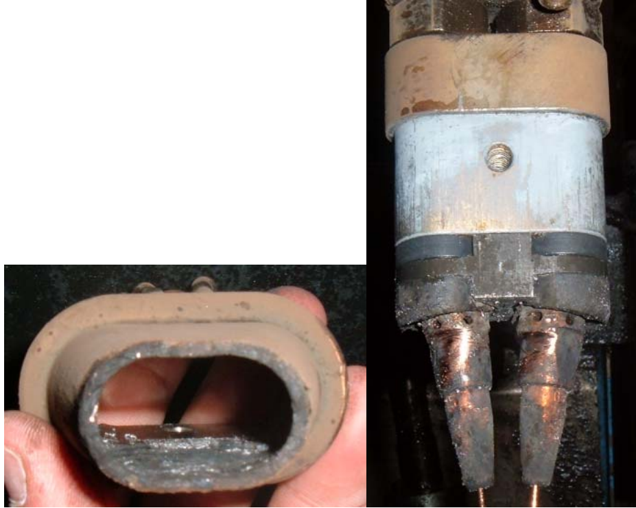
Cloos Nozzle, tips and diffusers after 120 parts with Intertech reamer.
