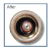
The IWE UltraCleaner is the first nonmechanical cleaner that can automatically remove spatter from any robotic GMAW torch including twin wire. The ultrasonic waves created in the anti-spatter fluid remove spatter from all torch components; including the contact tip, diffuser and nozzle. Longer consumable life is obtained because the UltraCleaner cools as it cleans.
